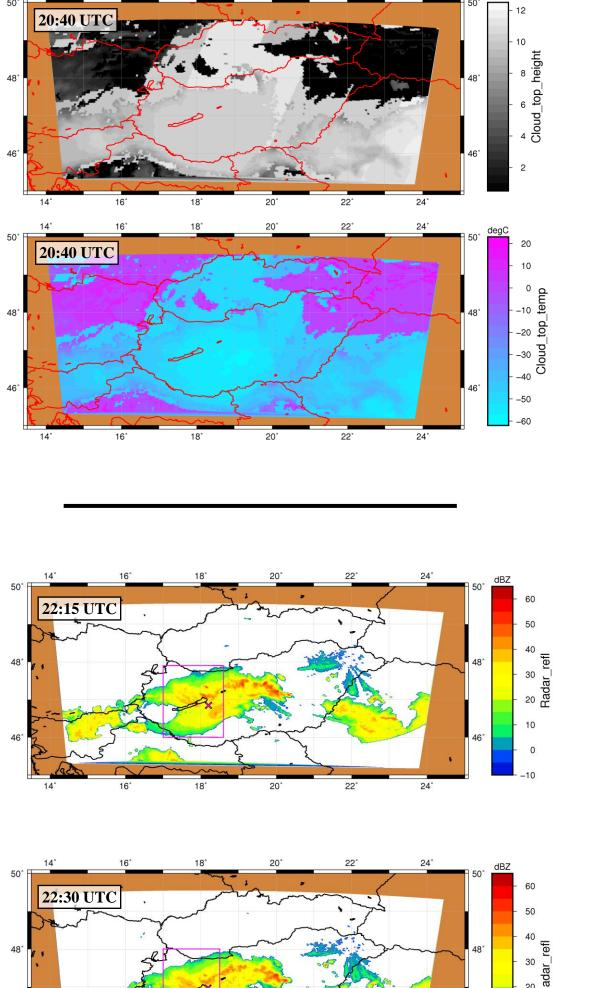
**Examples of sprite parent lightning stroke** locations on radar reflectivity maps
